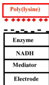
Scheme 1. Representation of the supramolecular structure (catalyst/ \text{Ca}^{2+} / \text{NAD}^+ /GDH/polylysine) at the modified glassy carbon electrode.
